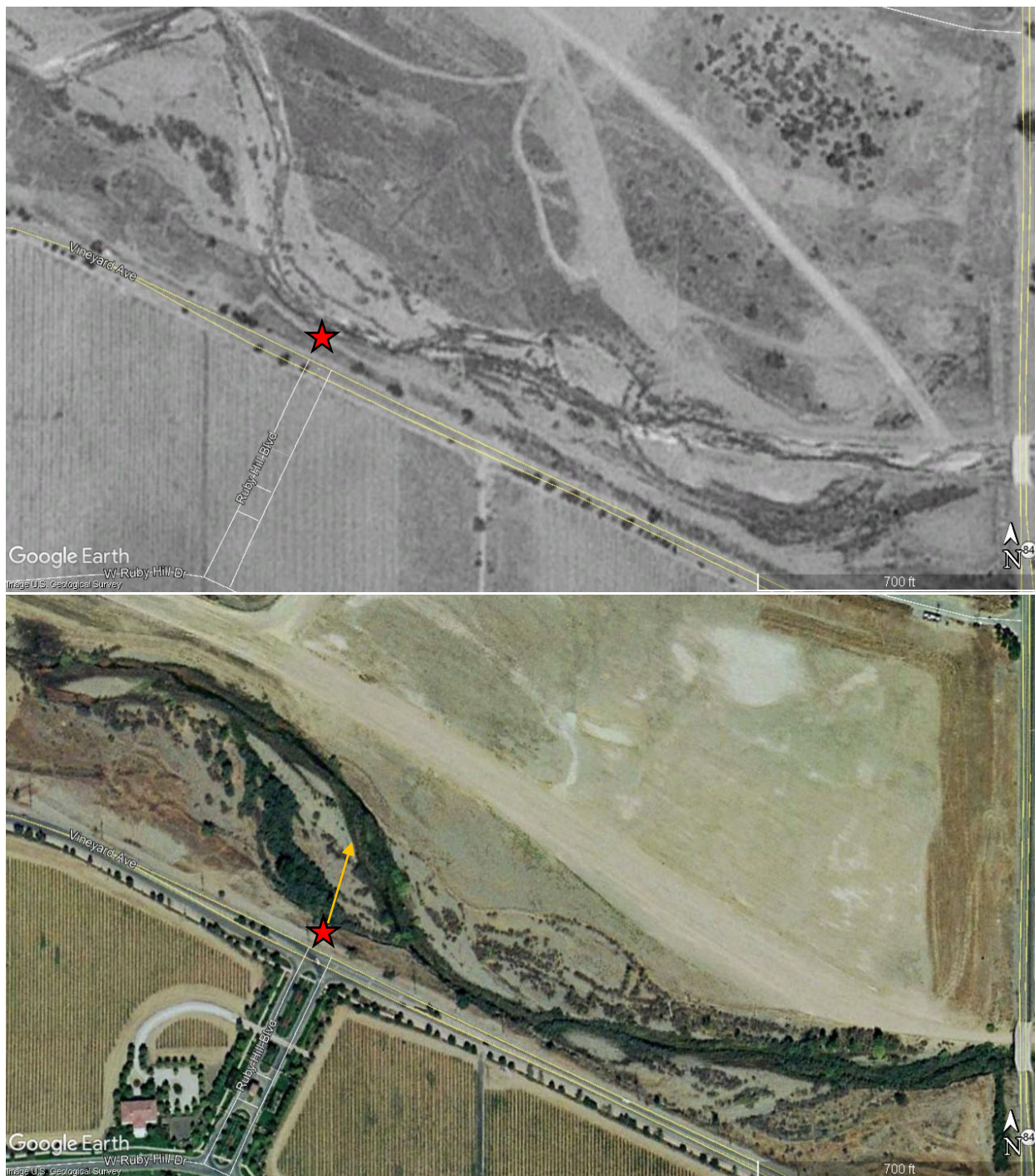
Figure 2. Google Earth aerial photos from 6/11/1993 and 10/30/2002 showing a multiple channel braided depositional system. The photo shows the area over the eastern portion of Lake B. Isabel Rd runs north-south along the right side of the photos. Over a ten year period the channel that was up against Vineyard Ave and the north point of Ruby Mill Blvd had been abandoned and the main channel was no 225' to the northeast.
